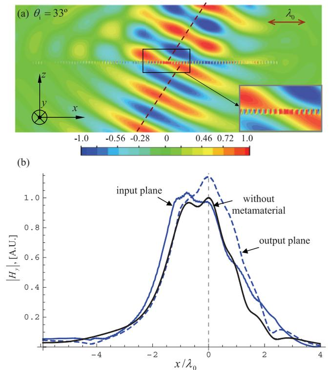
FIG. 5. (Color online) (a) Snapshot in time of the magnetic field  $H_y$  when the array of loaded wires is illuminated by a Gaussian beam with  $\theta_i = 33^\circ$ . The inset shows a zoom of the central region of the structure. (b) Amplitude of the magnetic field in arbitrary units (a.u.) calculated at (i) Solid blue curve: input plane, (ii) dashed blue curve: output plane, and (iii) black curve: similar to (i) but for propagation in free space.
