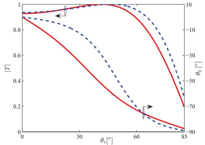
FIG. 4. (Color online) Discrete-loading model results of the transmission magnitude  $|T|$  and the transmission angle  $\theta_t$  as a function of the incidence angle  $\theta_i$  calculated at different frequencies. The red solid lines and blue dashed lines correspond to the results calculated at 10 GHz and 9 GHz, respectively.
