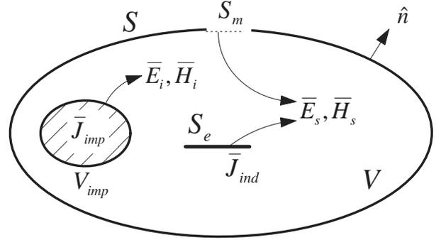
Fig. 3. Geometry of a closed-boundary waveguiding structure containing apertures and conducting strips in the presence of an impressed electric current source.
