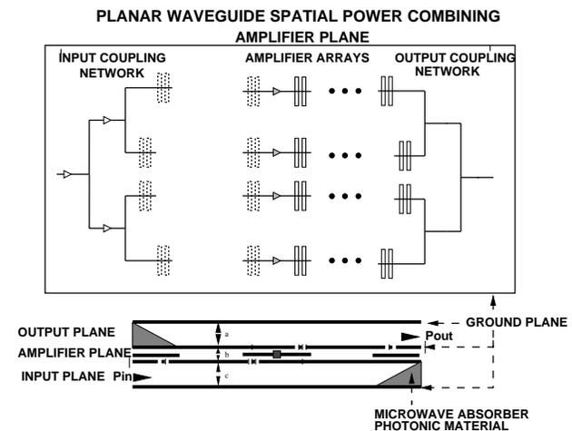
Fig. 2. Aperture-coupled planar waveguide amplifier array.
