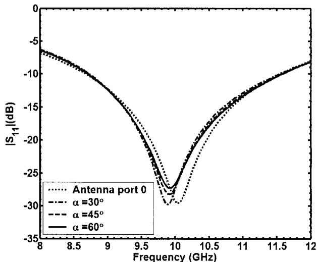
**Figure 5** Reflection coefficient of the bow-tie slot antenna fed with the tapered 50Ω CPW for different lengths of the tapered transition
