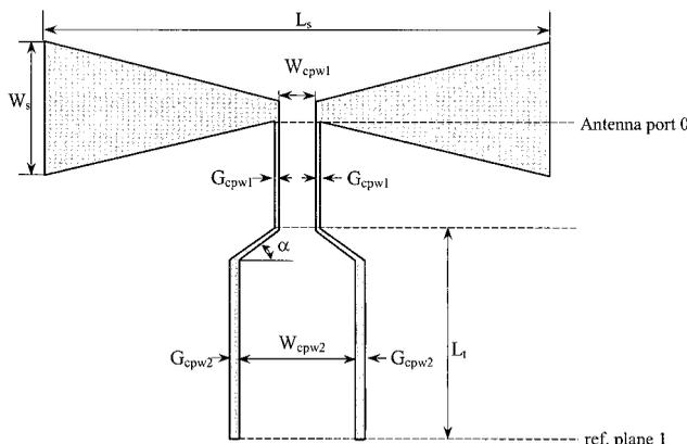
**Figure 3** Bow-tie slot antenna fed with the tapered CPW transition with  $W_{cpw2} = 3$ ,  $G_{cpw2} = 0.1650$ ,  $L_t = 10$ ,  $W_{cpw1} = 1.6548$ ,  $G_{cpw1} = 0.1$ ,  $L_s = 20.64$ ,  $W_s = 6.3$ , and  $\alpha = 45^\circ$  (dimensions in millimeters)
