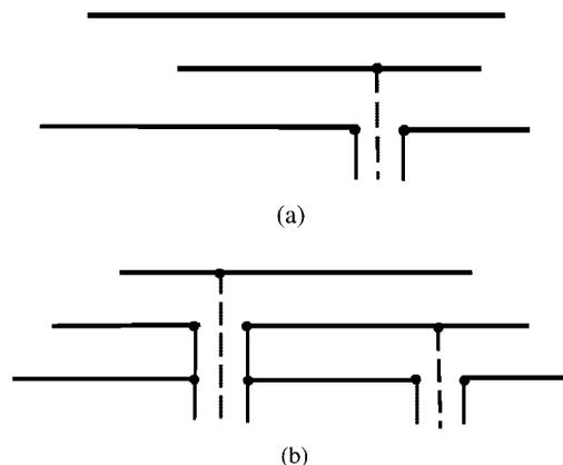
**Figure 1** (a) Single-feed stacked patch antenna for dual-frequency; (b) two-feed stacked patch antenna for dual-frequency
