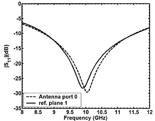
**Figure 4** Reflection coefficient calculated at the antenna port and reference plane 1 for the bow-tie slot antenna fed with the 50Ω tapered CPW transition
