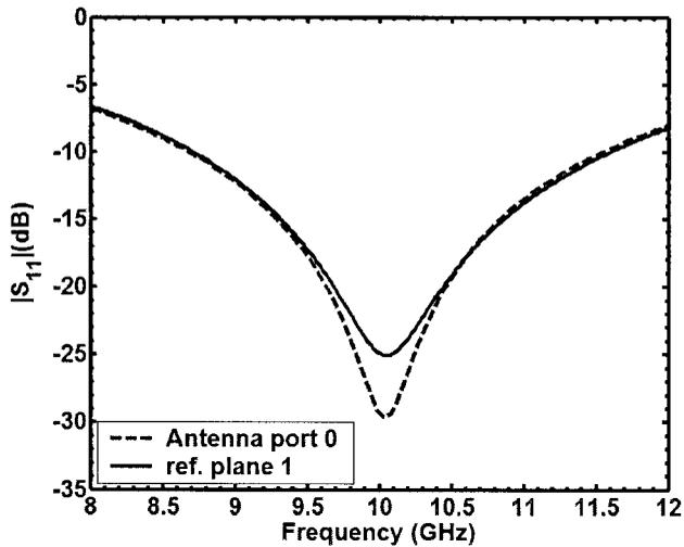
**Figure 2** Reflection coefficient at the antenna port and reference plane 1 for the bow-tie slot antenna fed with the 50Ω CPW
