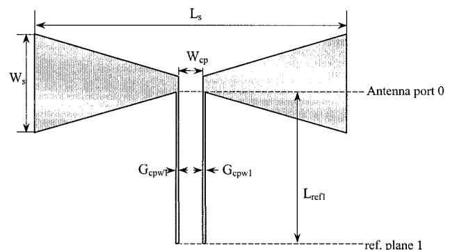
**Figure 1** Bow-tie slot antenna fed by the CPW line and different reference planes
