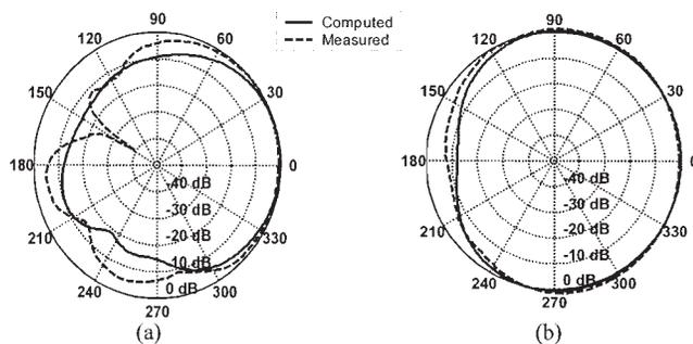
**Figure 3** Computed and measured radiation patterns for the printed bow-tie antenna at 10 GHz: (a) E-plane; (b) H-plane
