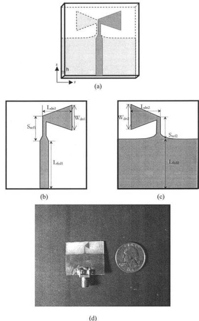
**Figure 1** Geometry of printed bow-tie antenna with a simplified feeding network: (a) 3D schematic view; (b) top layer; (c) bottom layer; and (d) photograph of the fabricated antenna
