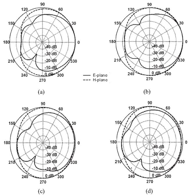
**Figure 4** Computed radiation patterns for the printed bow-tie antenna in the E-plane and H-plane: (a) 9 GHz; (b) 11 GHz; (c) 12 GHz; (d) 13 GHz
