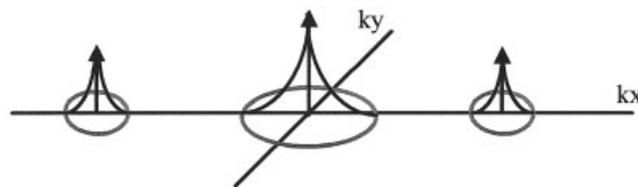
**Figure 2** Spectral representation of an off-axis hologram
