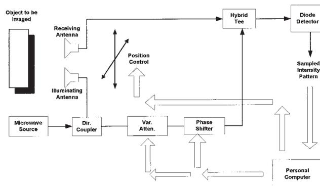
**Figure 1** Experimental arrangement for indirect microwave holographic imaging
