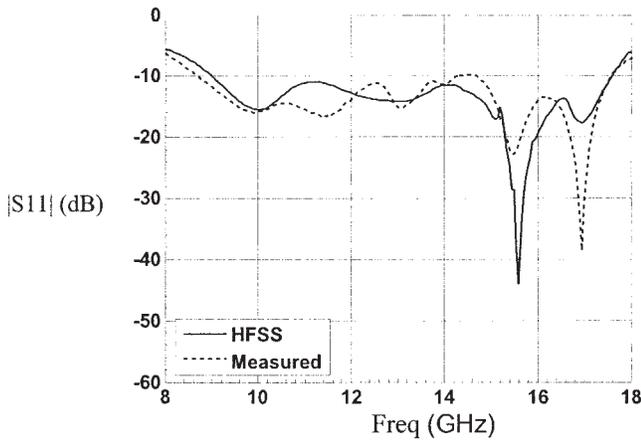
**Figure 2** Computed and measured reflection coefficients of the printed bow-tie antenna
