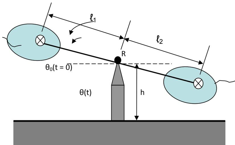
Fig. 2. Simplified termite model.
