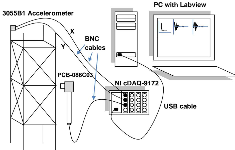
Fig. 2 Experimental setup
