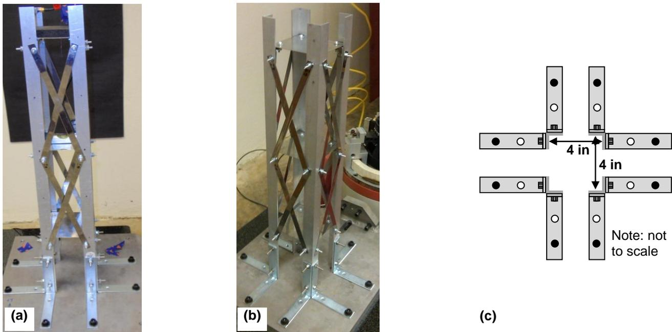
**Fig. 1** Three-story spatial frame structure (a) side view, (b) isometric view and (c) plan view
