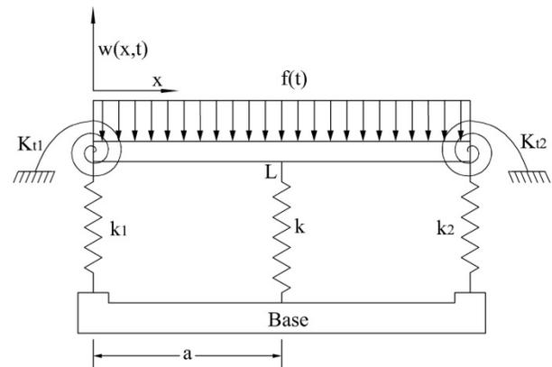
Figure 1. Beam model with adjustable boundary conditions and variable contact.
