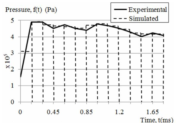
Figure 2. Example of force discretization with an experimental shock loading.
