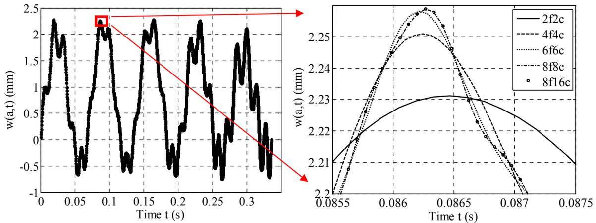
Figure 3. Convergence study for the reference case with fixed-free boundary conditions with an applied impulse of 0.1 milliseconds.
