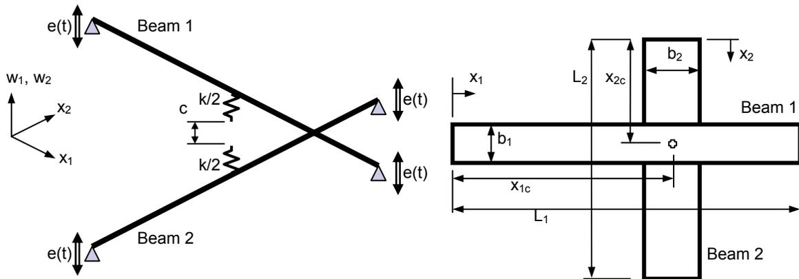
Figure 1. Two elastic beams that are subjected to base excitation and impact.
