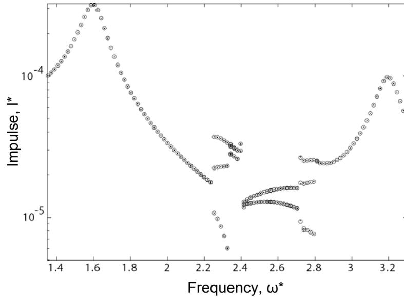
**Figure 2. Repetitive impact frequency response functions for the single beam model (---) and two beam model (ooo).**
