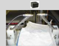
Resonant Ultrasound Spectroscopy Experiment to test Cement Paste
