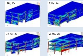
The response of a building to the removal of a column is analyzed using a three-dimensional finite element code. The building's resilience to an undesirable progressive failure is investigated and importance of shear walls on unintended slab and frame damage patterns observed.
