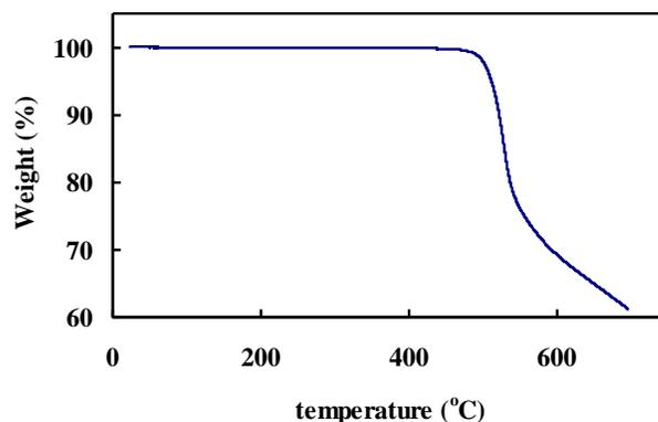
Figure 2. xGnP-PEI paper (MSU), in nitrogen, heating 10 °C/min.
