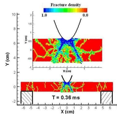
Impact on a 2D polymeric material body
