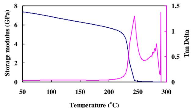
*Film tension, heating 10 °C/min, 1 Hz, in air.*
