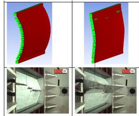
Numerical and experimental results for CMU wall retrofitted with polyurea
