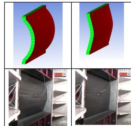
Numerical and experimental results for CMU wall retrofitted with POSS enhanced polyurea
