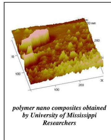
This work is at its initial stage. A graduate student is hired on this project and is being trained to use Nanoscope IIIa AFM. Topographic image of 2.5% MWCNT/Nylon 6,6 with tapping mode AFM was collected.
