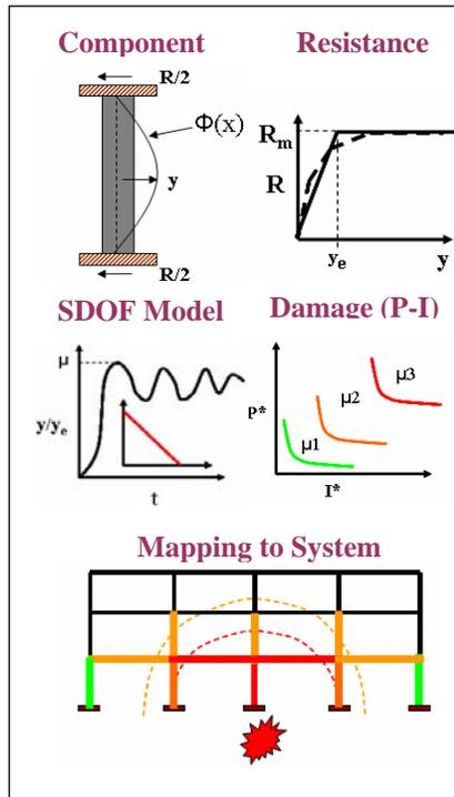
on the exposed column face, peak resistance for the minimum steel ratio case, natural period of SDOF oscillator, and effective yield displacement for SDOF oscillator.
