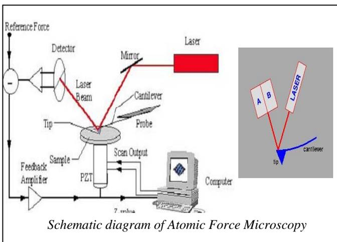
In this project, AFM is used as an imaging tool to evaluate the dispersion of nano particles in various matrices in order to study the topography of fractured surfaces and to get qualitative measure of particles adhesion. It will also be used to study local properties (modulus and hardness) of nano composites using indentation technique.
